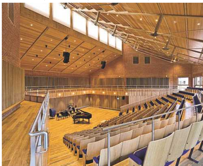
Bryanston School by Hopkins Architects – the simple and effective design of the moveable acoustic panels allows them to be adjusted manually
